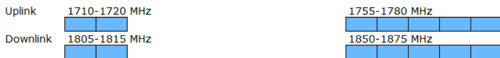
Figure 2 The figure shows the block division for the available frequency space in the 1800 MHz band
