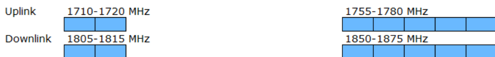
Figure 1 The figure shows the block division for the available frequency space in the 1800 MHz band
